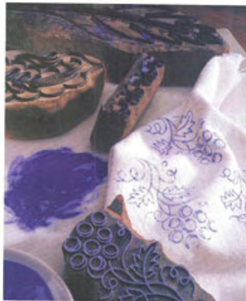
Stamping blocks- Metal strips imbedded in wood to form design. Block is dipped in thick solution and stenciled onto fabric.
